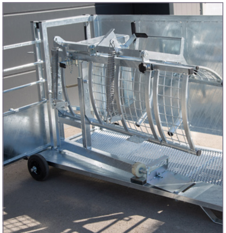
KM-JV-2-33 Hoof care crush with head bail / head gate
